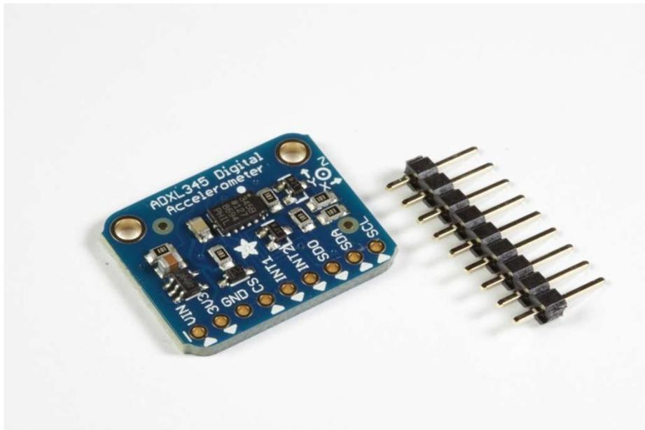
The ADXL345 is a low-power, 3-axis MEMS accelerometer modules with both I2C and SPI interfaces. The Adafruit Breakout boards for these modules feature on-board 3.3v voltage regulation and level shifting which makes them simple to interface with 5v microcontrollers such as the Arduino.
